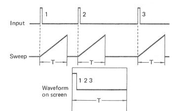
Fig. 12 Sweep in NORMAL sweep mode
