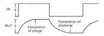
Fig. 3 In/output waveforms of a low-pass filter circuit
