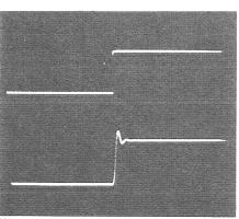
With capacitor,  $0.1\mu F$  (magnified:  $\times$  10)
