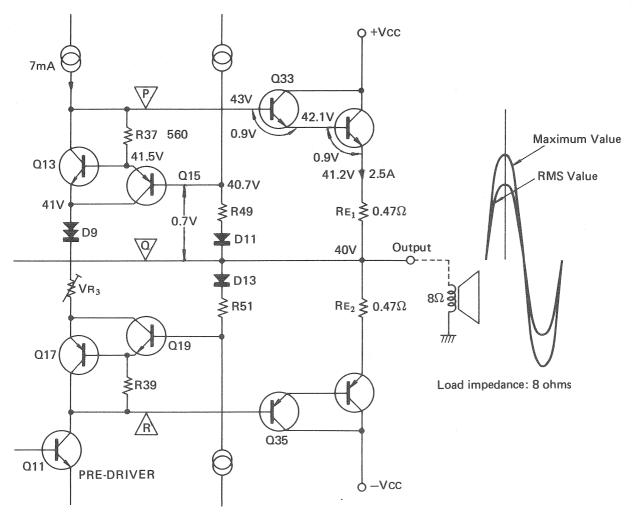
Fig. 10 Momentary potential at positive peak, 100W output
