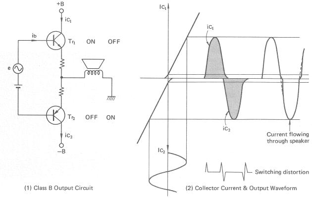
Fig 1 Generation of switching distortion
