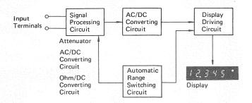
Fig. 1 Block diagram of digital multimeter
