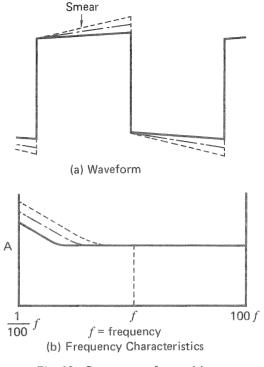
Fig. 10 Output waveform with smears
