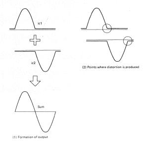
Fig. 20 In case collector currents are clear-cut
