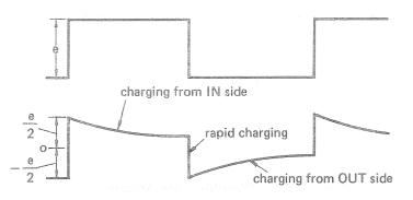
Fig. 5 In/output waveforms of High-pass filter circuit
