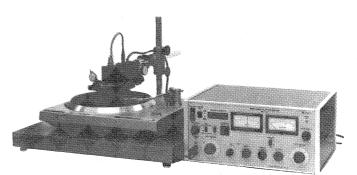
Photo 3 Wow/flutter measurement using rotary encoder
