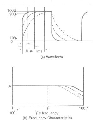
Fig. 7 Output waveform rise time
