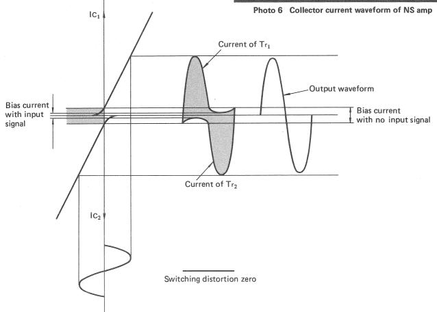
Fig. 7 Operation of Non-Switching amplifier
