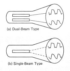
Fig. 9 Dual-beam & single-beam 'scopes
