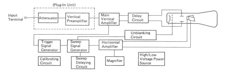
Fig. 8 Block diagram of trigger sweep 'scope
