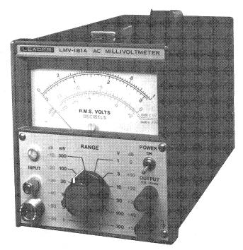
Photo 2 Use mV meter for audio signal measurement
