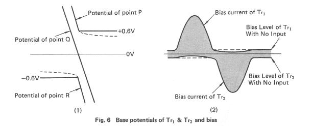
Fig. 6 (1) shows potential changes between the ground and points P, Q and R where the signal shifts from positive to negative. The bias levels of  $T_{r_2}$  when the signal is in positive half cycle, and of  $T_{r_2}$  when the signal is in negative half cycle, are not the same as those when no signal is present. The amplifier circuits are designed to reduce the bias levels slightly, as shown by the broken lines.
