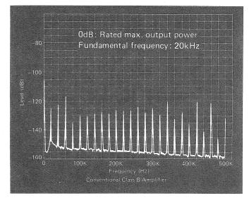
Photo 2 Distortion components
