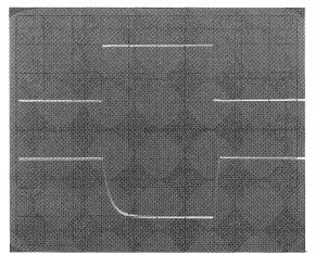
Photo 9-2 Conventional transistor switching characteristics
