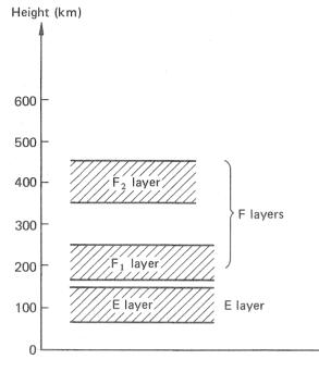
Fig. 6 "F" & "E" layers in earth's atmosphere
