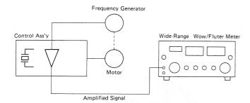
Fig. 7 Wow/flutter measurement with FG output direct-reading method
