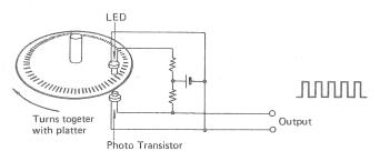
Fig. 6 Principle of rotary encoder
