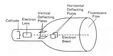
Fig. 1 Structure of cathode-ray tube
