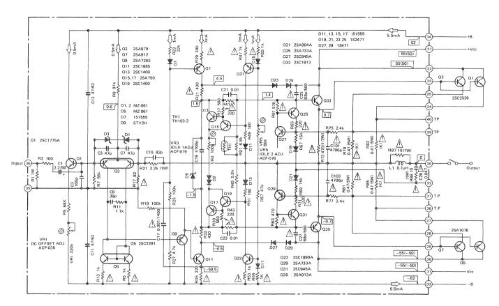
Fig. 8 Circuitry of SA-9800 Power Amp (Only left channel)
