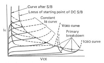
Fig. 3 Secondary breakdown phenomenon
