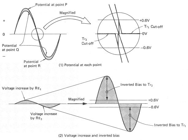
Fig. 5 Voltage drop by emitter resistors and cut-off
