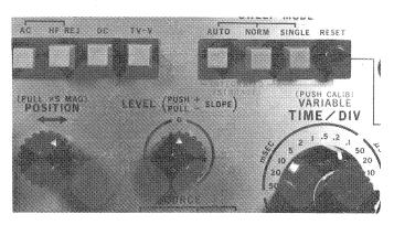
Photo 8 Trigger coupling and Sweep modes
