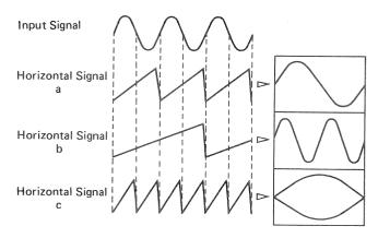
Fig. 5 Synchronization of repeating sweep type 'scope
