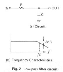
The circuit in Fig. 2 is low-pass filter represented by:  $fc = \frac{1}{2\pi Rc}$ .
