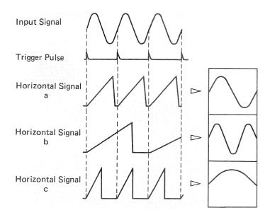
Fig. 6 Synchronization of trigger sweep type 'scope
