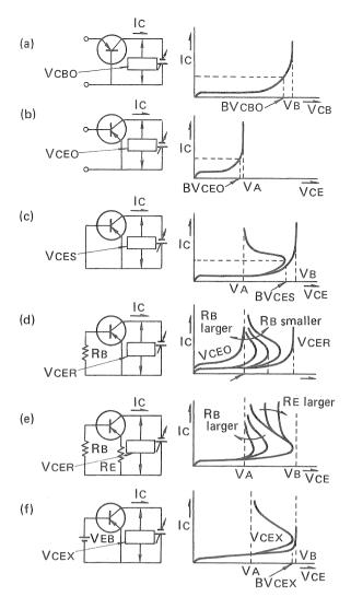
$\label{eq:VA} VA \mbox{=} avalanche \mbox{ breakdown voltage with emiter grounded } VB \mbox{=} avalanche \mbox{ breakdown voltage with base grounded }$
