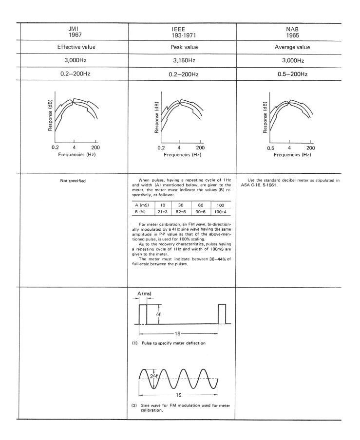
The existence of various standards for measuring wow/flutter makes comparison difficult. Each standard once had its own weighting curve. But DIN, that West German one with the most clear-cut regulations, was proposed to CCIR, an international standard council, as an international standard. CCIR adopted it in 1966.
