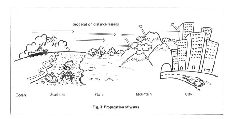
The lower the frequency of the surface wave, the longer its range. Radio waves with long wavelengths are, for this reason, used in long-range communications, such as for maritime purposes.
