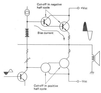
Fig 24. Load fluctuation of pre-driver in Class B
