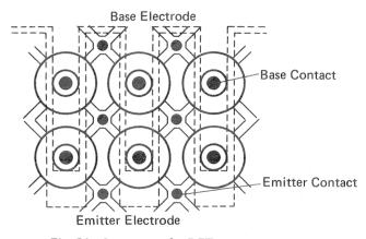
Fig. 21 Structure of a RET
