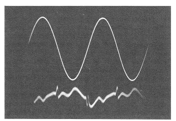
Photo 1 Output & distortion waveforms
