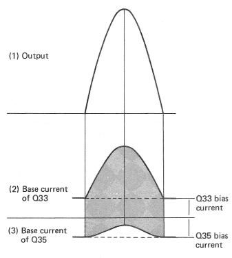
Fig. 14 Output and base current changes
