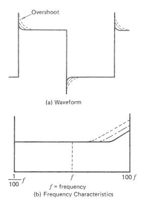
Fig. 9 Output waveform with overshoot
