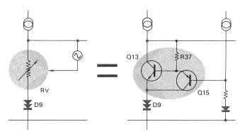
Fig. 11 Operation of Q13, Q17 & R37
