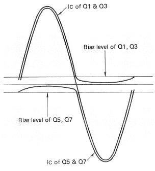
Fig. 19 Current waveform of output transistors
