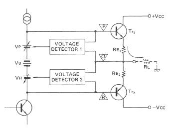
Fig. 4 Principle of Non-Switching amplifier
