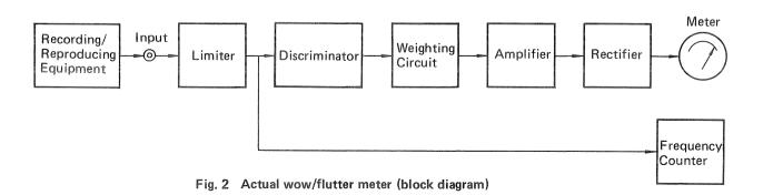
The human ear's sensitivity to sound level differs with frequency. Wow/flutter frequencies are low—in the area where human hearing is relatively insensitive. Therefore, in measuring wow/flutter, the measured value is compensated (weighted) to make the measuring instrument's response similar to a human's. This is achieved by raising the meter's response to those frequency components which are easily heard by the human ear, and by stepping down its response to those which are not.
