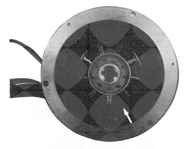
Photo 5 FG in Quartz-PLL DD motor
